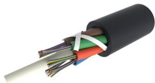
Fiber OSP cable, Zero Water Peak,<sup>®</sup> Blown Micro Single Jacket All-Dielectric Outdoor Stranded Loose Tube 200um Fiber Arid-Core™ Construction, 288 fiber, Singlemode G.652.D and G.657.A1, Gel-filled, Meters jacket marking, Black jacket color
