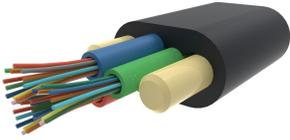
Fiber outdoor drop cable, LightScope® ZWP Self-Supporting All-Dielectric, Singlemode G.652.D and G.657.A1, Arid Core construction, Gel-filled, central loose tube, no ripcords, Feet jacket marking, Black jacket color
