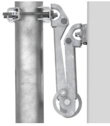
Wide Profile Antenna Downtilt Mounting Kit for 2.4 - 4.5 in (60 - 115 mm) OD round members. Kit contains one scissor top bracket set and one bottom bracket set.
