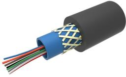
Fiber indoor/outdoor cable, LightScope® ZWP, Gel-Filled loose tube, Singlemode G.652.D, 6 fiber, meters jacket marking, Black jacket color, Dca flame rating
