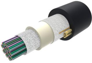
Fiber OSP cable, Non-Armored, All-Dielectric, Arid-Core, Dry Central Tube Rollable Ribbon, 288 fiber, 200um Singlemode G.652.D and G.657.A1, Gel-free, Feet jacket marking, Black jacket color
