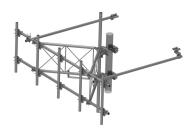
G23RHDXL PIM OPTIMIZED SPACING High Capacity Sector Frame with extended 10' Spine for RRU Mounting & extended frame for sites requiring increased sector to sector antenna spacing. 2 7/8in OD x 14.5ft face with (5) 2-7/8in OD x 96in Antenna pipes
