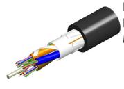
Fiber indoor/outdoor cable, LazrSPEED®, Light Duty, Single Jacket, Riser Rated, Gel-Free, All-Dielectric Outdoor Stranded Loose Tube, 6 fiber, Multimode OM3, Gel-free, Feet jacket marking, Black jacket color
