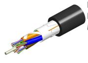
Fiber indoor/outdoor cable, LazrSPEED®, Light Duty, Single Jacket, Riser Rated, Gel-Free, , 12 fiberAll-Dielectric Outdoor Stranded Loose Tube, Multimode OM3, Gel-free, Feet jacket marking, Black jacket color
