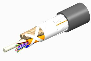
Fiber indoor/outdoor cable, TeraSPEED®, Single Jacket All-Dielectric, Plenum Rated, 36 fiber, Singlemode G.652.D and G.657.A1, Gel-Free, Stranded Loose Tube, PVDF jacket, Black jacket color, Feet cable marking
