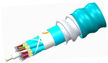
Fiber indoor cable, LazrSPEED® Riser/LSZH rated Distribution, interlocking aluminum armored, Multimode OM4, 6 fiber single-unit, Gel-free, Feet jacket marking, Aqua jacket color
