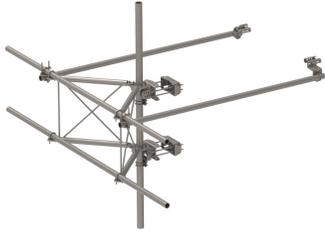
G23RHDX Tower Sector Frame with spine extension for RRU Mounting, 11 ft x 2.88 in OD face pipes. Base Kit Only. No antenna pipes.
