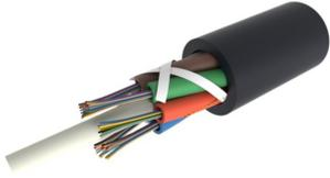
Fiber OSP cable, Zero Water Peak,<sup>®</sup> Blown Micro Single Jacket All-Dielectric Outdoor Stranded Loose Tube 200um Fiber Arid-Core™ Construction, 192 fiber, Singlemode G.652.D and G.657.A1, Gel-filled, Meters jacket marking, Black jacket color
