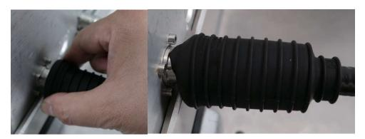
Twist and push up the swollen part of the boot severial times until the boot stretches to cover the female neck.
