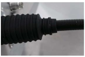
Push the conduit and stopped by gasket and ensure conduit is fully cover the gasket.
