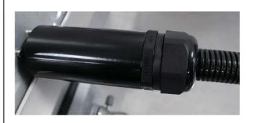
Do not hold the connector and bend the cable directly behind it, start bend 30mm min away from the cap end as picture shown.
