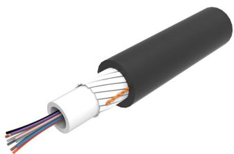
Indoor/Outdoor Low Smoke Zero Halogen, LazrSPEED® Central Loose Tube Fiber Optic Cable, 4-fiber, Multimode OM5, Gel-free, black. Provides Rodent Resistance.
