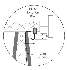
**Reminder:** Plan grip location by measuring distance (D) from Fiber Enclosure Box to tower support member.
