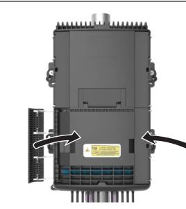
Once all cables are connected and properly secured, close the junction box and fasten all closures as instructed in the provided HFDC installation guide. Double-check that everything is secure to prevent environmental damage or tampering. Inspect the installation to ensure the box is properly mounted, and cables are managed without kinks or bends.
