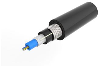
Fiber Indoor/Outdoor cable, TeraSPEED®, 120 min Fire Survival, Low Smoke Zero Halogen (LSZH), 12 fiber, Gel-Filled, Central Loose Tube, Singlemode G.652.D and G.657.A1, Meters jacket marking, Black jacket color. Provides Rodent Resistance.
