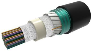
Fiber OSP cable, Armored, Arid-Core, Dry Central Tube Rollable Ribbon, 288 fiber, Singlemode G.652.D and G.657.A1, Gel-free, Feet jacket marking, Black jacket color
