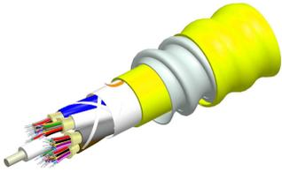
Fiber Indoor cable, TeraSPEED® Riser Distribution, interlocking aluminum armored with riser jacket, 2 fiber single-unit, Gel-free, Singlemode G.652.D and G.657.A1, Feet jacket marking, Yellow jacket color
