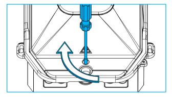
1 Secure by turning the locking screw clockwise.
