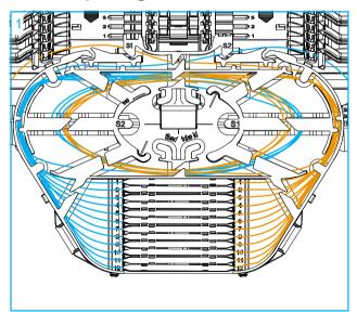
1 Make splice per local practice and store the splice protector in the splice protector holder. Store the over lengths in loops in the over length storage area.
