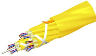
Fiber indoor cable, Plenum MPO Trunk Cable, 144 fiber with 24-fiber, 3.0 mm subunits, Gel-free, Singlemode G.657.A2, Feet jacket marking, Yellow jacket color
