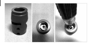
With the back of the tool on a flat surface, push the coring blade assembly from the tool using a Philips screw driver placed in the center hole of the tool. Do not hit or press on the edge of the coring blade. All force should be applied to the center of the assembly only.
