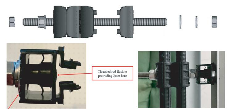
NOTE: Critical to maintain a tightening torque between 3-5Nm. Failure to do so will adversely affect hanger performance.
