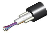
Fiber Indoor/Outdoor cable, Single Jacket Gel-Filled All-Dielectric Riser Rated Central Tube, 24 fibers, Singlemode G.657.A2, Feet jacket marking, Black jacket color
