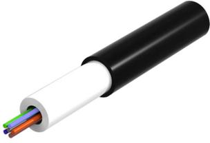
Fiber OSP cable, LightScope® ZWP Blown Single Jacket All-Dielectric Outdoor Central Tube Construction, Singlemode G.652.D and G.657.A1, 24 fiber, Gel-filled, Meters jacket marking, Black jacket color and fiber color as per TDC-TS 900 011a RM: 50-75mm
