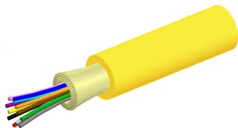
Fiber indoor cable, LSZH Riser Rollable Ribbon Dual Rated Backbone, 36 fiber, Singlemode G.657.A2/B2, Feet jacket marking, Yellow jacket color, Cca flame rating
