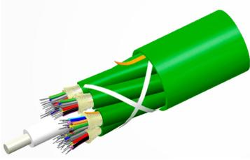
Fiber indoor cable, LazrSPEED® Plenum Distribution, 36-Fiber Multi-Unit with 12-Fiber Subunits, Multimode OM3, Gel-free, Feet jacket marking, Green jacket color
