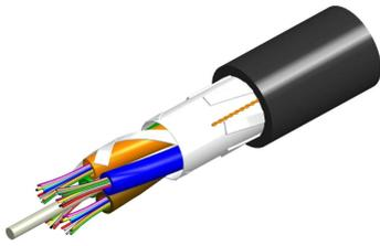
Fiber OSP cable, LightScope® ZWP Single Jacket All-Dielectric, 12 fiber, Gel-Free, Stranded Loose Tube, Singlemode G.652.D and G.657.A1, Feet jacket marking, Black jacket color
