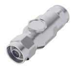
Arrestor Gas Tube Surge Arrestor (350 V), 2400–2500 MHz, with interface types N male for 1/2" Superflexible Foam Coaxial Cable
