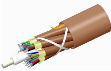
Fiber indoor cable, TeraSPEED® Plenum Distribution, 144 fiber multi-unit with 12 fiber subunits, Singlemode G.652.D and G.657.A1, Gel-free, Feet jacket marking, Brown jacket color
