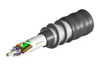
Fiber indoor/outdoor cable, TeraSPEED®, Plenum Rated, Singlemode G. 652.D and G.657.A1, Gel-Free, 72 fiber, Stranded Loose Tube with Aluminum Interlocking Armor containing a Plenum Rated Outer Jacket, Black jacket color, Feet cable marking
