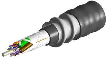
Fiber indoor/outdoor cable, LazrSPEED®, Plenum Rated, Gel-Free, Stranded Loose Tube with Aluminum Interlocking Armor containing a Plenum Rated Outer Jacket, 12 fiber, Multimode OM3, Feet jacket marking, Black jacket color
