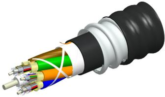
Fiber indoor/outdoor cable, TeraSPEED® LSZH Riser Distribution, interlocking aluminum armored, 6 fiber single-unit, Singlemode G.652.D and G.657.A1, Feet jacket marking, Black jacket color
