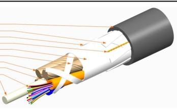
Plenum-Rated Outer Jacket Strength Elements Binder Water Swellable Tape Ripcord (1) Binder 2.5 mm Gel-Free Buffer Tubes 250 micron Fibers Dielectric Strength Member
