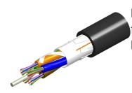
Fiber OSP cable, TeraSPEED® Light Duty, Single Jacket, All-Dielectric, 2 fiber, Gel-Free, Stranded Loose Tube, Singlemode G.652.D and G.657.Al, Feet jacket marking, Black jacket color
