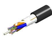
Fiber OSP cable, LazrSPEED®, Light Duty, Single Jacket, All-Dielectric, Gel-Free, Stranded Loose Tube, 2-fiber, Multimode OM3, Feet jacket marking, Black jacket color
