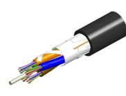
Fiber OSP cable, LazrSPEED®, Light Duty, Single Jacket, All-Dielectric, Gel-Free, Stranded Loose Tube, 2-fiber, Multimode OM4, Feet jacket marking, Black jacket color
