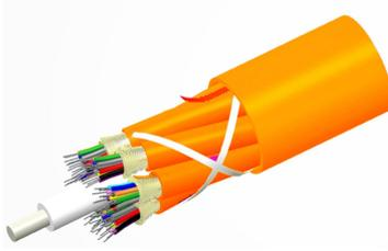
Fiber indoor cable, TeraSPEED® Plenum Distribution, 48 fiber multi-unit with 12 fiber subunits, Composite OM3 and G.652.D and G.657.A1, Gel-free, Feet jacket marking, Orange jacket color
