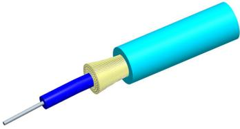
Fiber Indoor Cable, LazrSPEED® 1.6mm Low Smoke Zero Halogen Riser, 1-fiber Simplex, Multimode OM4, Feet jacket marking, Aqua jacket color, Eca Flame Rating
