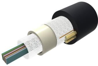
Fiber indoor/outdoor Cable, LSZH Riser All-Dielectric Central Tube Ribbon, Multimode OM3 bend insensitive, 96-fiber, feet jacket marking, black jacket color
