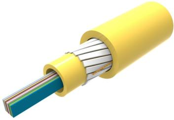
Fiber Indoor Cable, LSZH Riser, All-Dielectric, Central Tube Ribbon, Singlemode, G.652.D and G.657.A1, 72 Fibers, Gel-free, Feet jacket marking, Yellow jacket color
