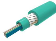
Fiber Indoor Cable, LSZH Riser, All-Dielectric, Central Tube Ribbon, Multimode, OM4, bend insensitive, 48 Fibers, Gel-free, Feet jacket marking, Aqua jacket color
