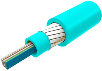
Fiber Indoor Cable, LSZH Riser, All-Dielectric, Central Tube Ribbon, Multimode, OM4, bend insensitive, 60 Fibers, Gel-free, Feet jacket marking, Aqua jacket color
