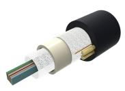
Fiber OSP Cable, Non-Armored, All-Dielectric, Arid-Core, 96 fiber, Dry Central Tube Ribbon, Singlemode G.652.D and G.657.Al, Gel-free, Feet jacket marking, Black jacket color
