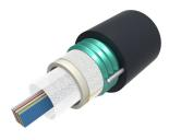
Fiber OSP cable, Steel Armored, Arid-Core, Dry Central Tube Ribbon, Multimode OM4, bend insensitive, Feet jacket marking, Black jacket color
