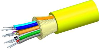
Fiber indoor cable, LazrSPEED® Plenum Distribution, 12 fiber single-unit, Multimode OM4, Feet jacket marking, Yellow jacket color
