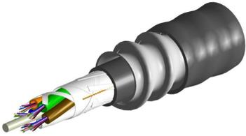
Fiber indoor/outdoor cable, TeraSPEED® Inner LSZH, Mini Stranded Loose Tube, Riser Rated, 36 fiber, Singlemode G.652.D and G.657.A1, Gel-Filled Subunits, Aluminum Interlocking Armor, Black jacket color, Feet jacket marking
