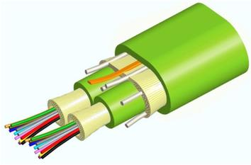
Fiber indoor cable, LazrSPEED®, Low Smoke Zero Halogen Riser MPO Trunk, 24 fiber with 12 fiber subunits, Gel-free, Multimode OM5, Feet jacket marking, Lime green jacket color, Dca flame rating
