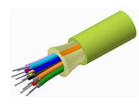
Fiber indoor cable, LazrSPEED® Riser Distribution, 24-Fiber Single-Unit, Multimode OM5, Feet jacket marking, Lime green jacket color
