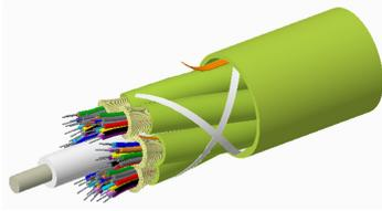
Fiber indoor cable, LazrSPEED® Riser Distribution, 144 fiber Multi-Unit with 12-Fiber Subunits, Multimode OM5, Gel-free, Feet jacket marking, Lime green jacket color
